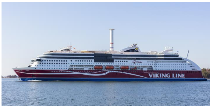
Viking Grace after installation of the 24x4 Rotor Sail.
