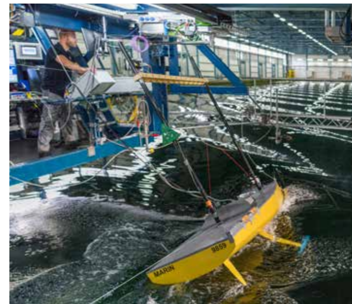
V065 model in waves in the basin
