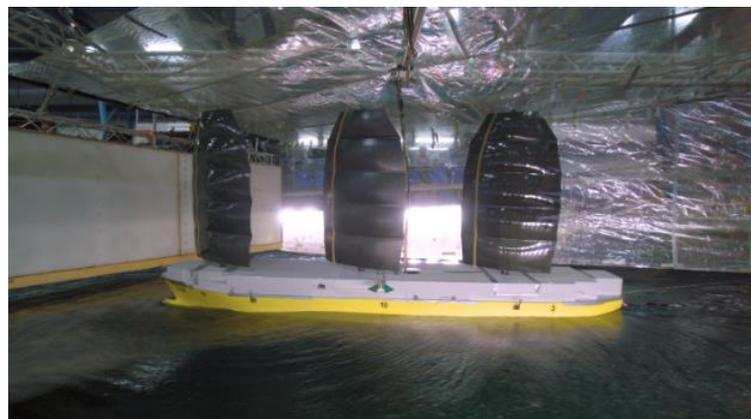
tunnel. The test set-up was evaluated regarding its usefulness and accuracy. Calculations were done in parallel to quantify the impact of some simplifications adopted in the test set-up. The test results indeed indicate that the seakeeping and manoeuvring behaviour of ships change wind assistance. Besides this novel test set-up, the alternative set-up of applying aerodynamic forces with dynamically controlled winches in a basin test remains practical to use.
