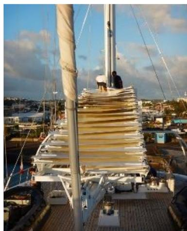
**Chantiers De L'Atlantique** is completing its successful trial session of SOLID SAIL started October 2018 onboard Le Ponant. In parallel, the development program is going on to introduce lessons learnt in the frame of this one year full test at real scale of SOLID SAIL and a platform test will be installed in September in Chantiers de l'Atlantique to finalize the development and show the product to the community, including ship owners, engineering offices and naval architects.
