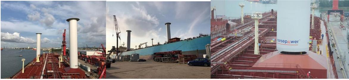
**Norsepower (Finland) - Wind Propulsion First – Installation of 2 x 30m Rotorsails on 109,000dwt Maersk Pelican LR2 product tanker**, estimated to save 7-10% fuel. Another great stride forward in commercial wind propulsion installation. <https://youtu.be/7fjS-lLVoA> <https://www.norsepower.com/news>
