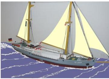
**SS Eileen II (Germany) - Offshore supply vessel concept:** Based on the development of the sailing coaster *SS Eileen* with little alterations in specific features, the team is looking at the offshore supply vessel market. An intelligent combination of conventional rigging with modern technologies without expensive pre-development results in an energy-efficient way to serve even supply tasks in coastal operation areas. <http://wind-ship.org/en/schormanns-maritima-iwsa-associate-member/>
