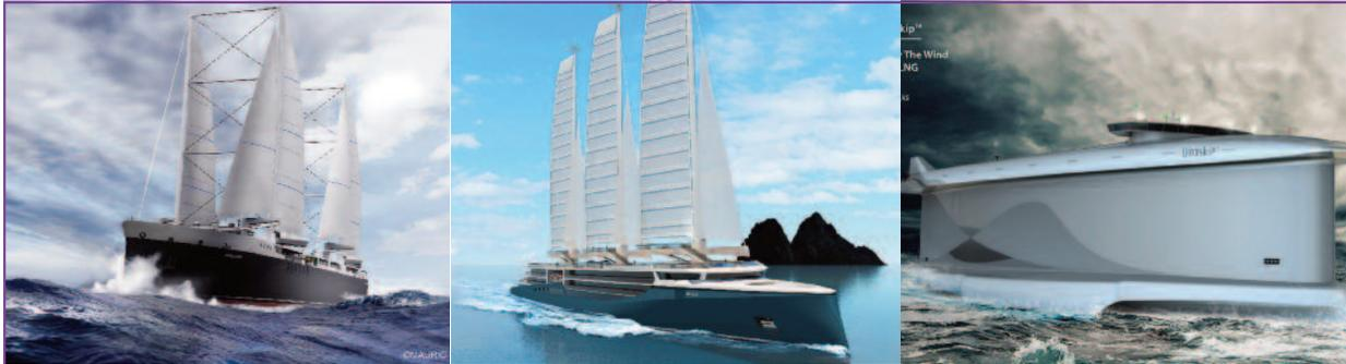
**Figure 3.** Primary Wind Designs: (left) Neoliner 136m Roro, (center) Silenseas 210m Cruise vessel (Chantiers de l'Atlantique), and (right) Vindskip Car Carrier Design.
