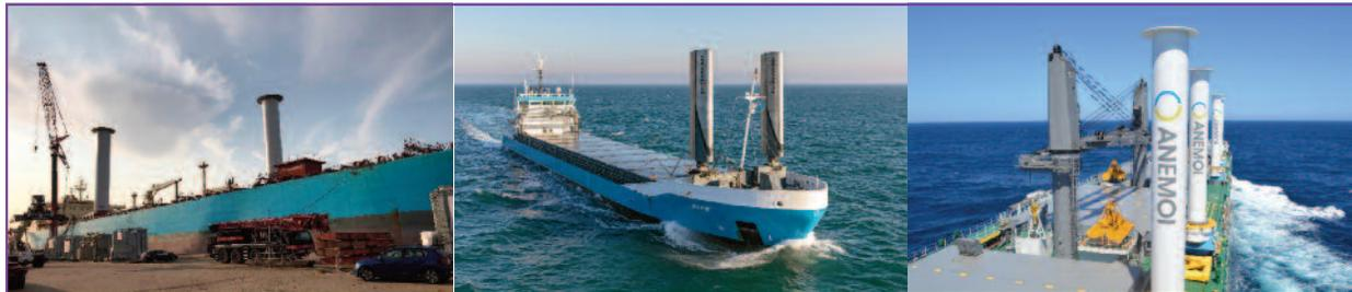
**Figure 2.** Example installations: (left) Maersk Pelican, 109,000dwt LR2 Tanker (2 x 30m Norsepower Rotors); (center) MV Ankie, 3,600 dwt (2 x 10m collapsible Econowind Ventifoil Suction Wings); and (right) MV Afros, 64,000dwt Geared Bulker (4 x movable Anemoi Rotors).
