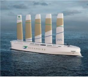
[Wallenius Marine](#) & Alfa Laval have formalised their 50/50 joint venture, known as AlfaWall Oceanbird with Niclas Dahl as its new managing director. The Oceanbird concept is to install wing sails on a transatlantic car carrier with a capacity of 7,000 vehicles. The solution should cut emissions by up to 90% compared to today's most energy-efficient vessels at an average speed of 10 knots. [Read more...](#)
