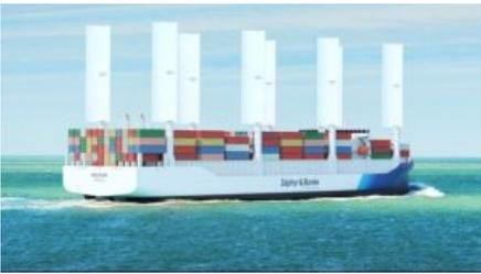
[Zéphyr & Borée](#) has been awarded Approval in Principle (AiP) by [Bureau Veritas](#) for its first wind-assist open-top 185m, 1,800 TEU containership. Propulsion means are compliant with IMO's Tier III requirements, and the vessel is equipped with shaft generators and a heat recovery system to minimize fuel consumption. The vessel's propulsion system will be assisted by eight sails provided by [Computed Wing Sails \(CWS\)](#).
