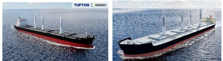
In May, [ANEMOI Marine Technologies](#) announced a project with Tufton Investment Management to install 3 large Rotor Sails on their TR Lady, a 82,000DWT Kamsarmax bulker due in mid-2022, will see Anemoi installing the Rotor Sails on their unique rail deployment system, allowing rotors to be moved during cargo operations. [Read more...](#)
