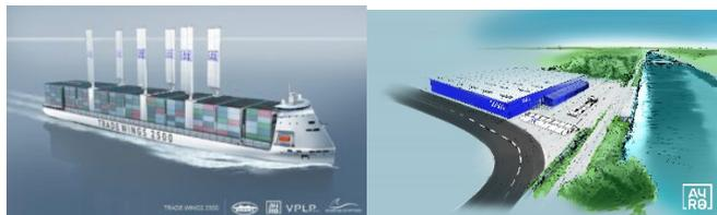
[AYRO](#) announced in May that their new wind-assisted containership design, the Trade Wings 2,500 has received an AiP from [Bureau Veritas Group](#). The vessel, which has been designed jointly by [VPLP](#) design, Alwena Shipping, SDARI and [AYRO](#), features six Oceanwing wingsails installed on a vertical sliding mechanism so they can be retracted partially while the vessel is in port. The wingsails alone will deliver c.20% of the total propulsive energy for the vessel. [Read more...](#)
