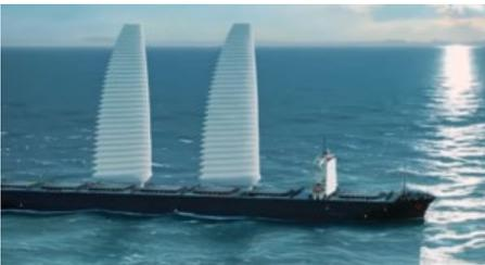
[Michelin](#) announced the development of the inflatable WISAMO (WIng SAIL MObility) which is projected to improve ship fuel efficiency by up to 20%.
