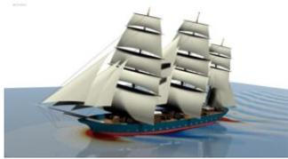
[Cape Horn Engineering Ltd.](#) and [EcoClipper](#) have partnered up to push the Ecoclipper 500 vessel design work to the next level. Extensive CFD simulations for 4 different candidate hulls were performed and compared at different sailing conditions to aid the design process. [Read More...](#)
