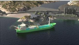
**Northern Lights:** Shell's joint venture with energy majors Equinor and TotalEnergies, has placed an order for two, 130m long LNG-powered, wind-assisted CO2 carriers, with a 7,500m3 capacity at China's Dalian Shipbuilding Industry Co. (DSIC) to be delivered in mid-2024. [Read more...](#)
