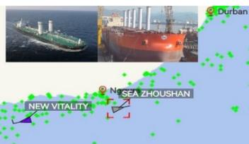
**A Historic Moment** - the two largest wind-assist vessels in the world meet off the coast of South Africa for the first time. The newly launched VLOC bulk carrier Sea Zhoushan chartered by Vale with five rotor sails in operation and the VLCC tanker, New Vitality operated by China Merchants Energy Shipping Co., Ltd. (CMES) and fitted with two retractable rigid sails.
