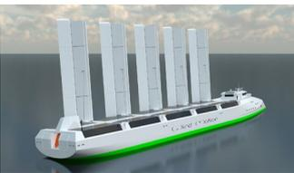
**Wind Motion 120 AFS:** The most efficient passive wing (non-motor assisted) has an Asymmetric profile, with adjustable Flap and Slat (AFS) This project investigates the feasibility for ships to optimally operate such wings, for 100% wind propulsion target. More details here: [Mathis Rühl Naval Architecture](#)
