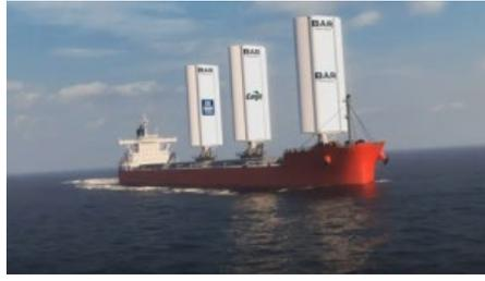
[BAR Technologies](#) AiP from DNV has been awarded to BAR Technologies for their WindWings system ahead of the first installation of the system in 2022, and deployment as part of the EU Horizon CHEK research project. [Read more...](#)
