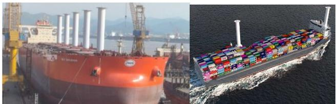
[Norsepower](#) celebrated the launch of the newly built MV Sea Zhoushan, a 325,000 dwt VLOC bulker with five of their tiltable rotor sails installed. The vessel is owned by Pan Ocean Ship Management and chartered by Brazilian mining company Vale. The rotor sails will deliver an estimate average yearly saving of 8% (based on a motor vessel operation) [Read more...](#)
