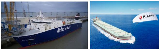
[Airseas](#) installed a 500m<sup>2</sup> version of their Seawing kite system on the 154m, 21,500 GT RoRo vessel, the MV Ville de Bordeaux owned by [Louis Dreyfus Armateurs](#) and chartered by Airbus in La Rochelle in December, and will undergo extensive testing from January.
