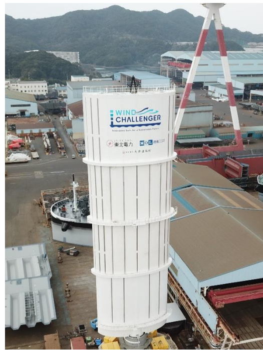
"Hard Sail for Wind Challenger" Left: Shortened Hard Sail Right: Extended Hard Sail
