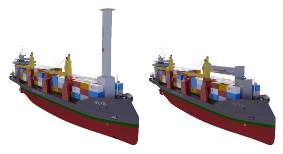
Rotor is located in the fore part of the vessel. A reinforcement of the hatches was done where the rotor foundation is fixed. Folding the rotor is an option available when this is needed in port or in navigation.
