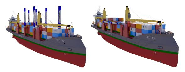
For the payload impact, the number of containers that must be removed from the main deck to use this alternative is 13 TEUs.
